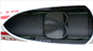
Image 1: Seat is too far forward. Nose would be down when static
